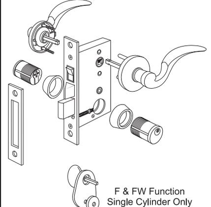
1. Position knob/plate or knob/rose assemblies on each side of door as shown. Make sure spindles from both sides are engaged with lock properly. Loosely tighten mounting screws.
