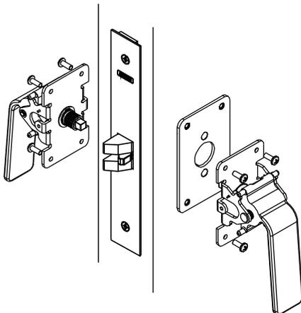
1. From outside of door, push outside mounting plate assembly through the door and lock body then from inside of door, place inside mounting plate on door and secure with 2 thru-bolt mounting screws.
