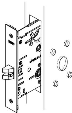
2. Insert lock and fasten with two screws.
