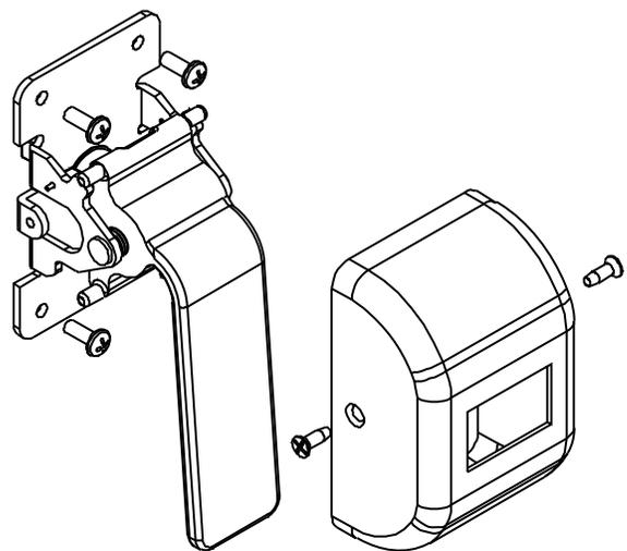
Assemble cover plates on inside and outside push/pull assemblies. Secure with two screws.
